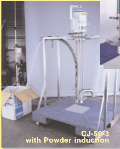
CJ-50-3 With Powder-Induction Device shown with induction tube drawing a carbomer powder directly out of a container bag.
